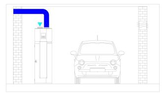
Installation with an intake duct and free expulsion is recommended if there is a desire to use the air expelled by the unit, cold dehumidified air  $(5-10^{\circ}C \text{ colder than the intake air})$ , to cool the room.
