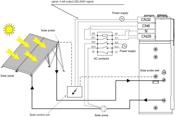
When the solar control unit check the temperature is OK in solar panel, it will output 220-240V signal.
