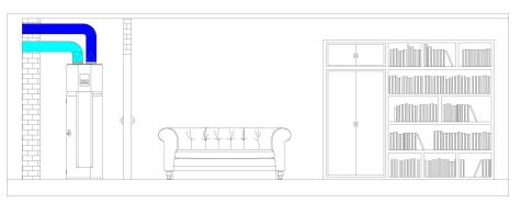
Channelling the intake and expulsion through ducts allows the unit to function with air taken from outside the house. Heat is extracted from the outdoor air, and used as a source for the heat pump.
